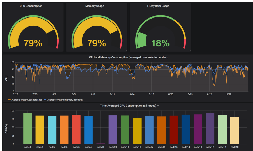
91 92 93 Fig. 1. Prometheus monitoring showing resource usage for one of the Kubernetes clusters
