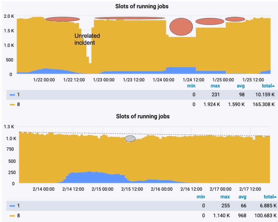
Fig. 3. CPU usage on the CERN Kubernetes cluster with the default scheduling algorithm (top) vs the node-packing policy (bottom). Resources that are unused due to inefficient scheduling are indicated with red ellipses. Also note the cluster size decreased from 2000 cores to 1000 cores, due to issues with the csi-cvmfs driver and the infrastructure at CERN, which were addressed at the time.
